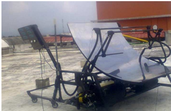
Fig 1 .Experimental setup of a parabolic trough collector
